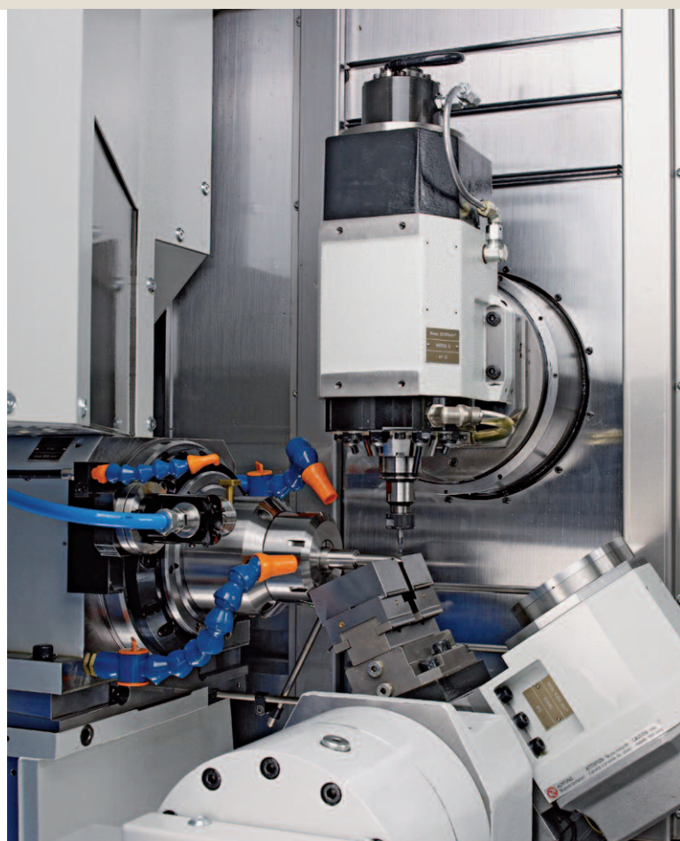
Figure 1. Turning, milling, drilling: With between five and eight CNC axes, turning and milling centres from Willemin-Macodel enable complete machining for micro components
