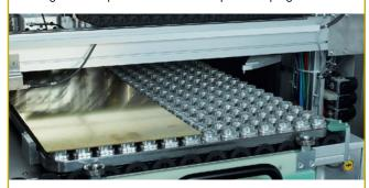
Removable: allows part handling out of the machine, e.g. with loader
