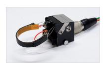
**Heating objective ring:** The Controller is specifically designed to slowly heat the objective over a fifteen minute warm-up period then hold the objective at the set point value within 0.2 °C. It operates from ambient to 50 °C. Special safety circuitry is utilized with a 0.9 °C error window. If for any reason the temperature of the objective deviates after it has reached set point, the controller shuts down and sounds an alarm. The Control unit is available at *piezosystem jena*.
